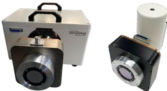
Closed-cycle cryocooler STU (left) and LN<sub>2</sub> pour-fill Dewar (right)
